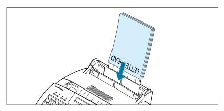
4. Slide both paper adjusters to fit against the paper's edges. **Ensure** the paper line flat in the tray.
